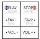
AP mode - in this mode it is possible to connect to the controller WIFI and log in to the existing WIFI network Every 3 seconds, PLAY and STOP flash at the same time
