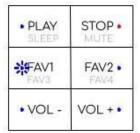
The controller is connected in to WIFI network, but could not find a paired LinkPlay player FAV1 flashes every 3 seconds
